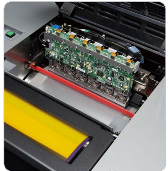
The Presstek 34DI incorporates 6 multi-beam laser diodes on each of its imaging modules.
